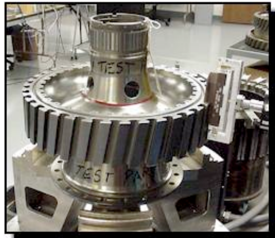
A probe begins the surface inspection of a disk using the Eddy Current Inspection Station. (Photo Courtesy of Veridian)
